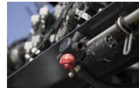
John Deere M-Spray a INC (Individual Nozzle Control)
